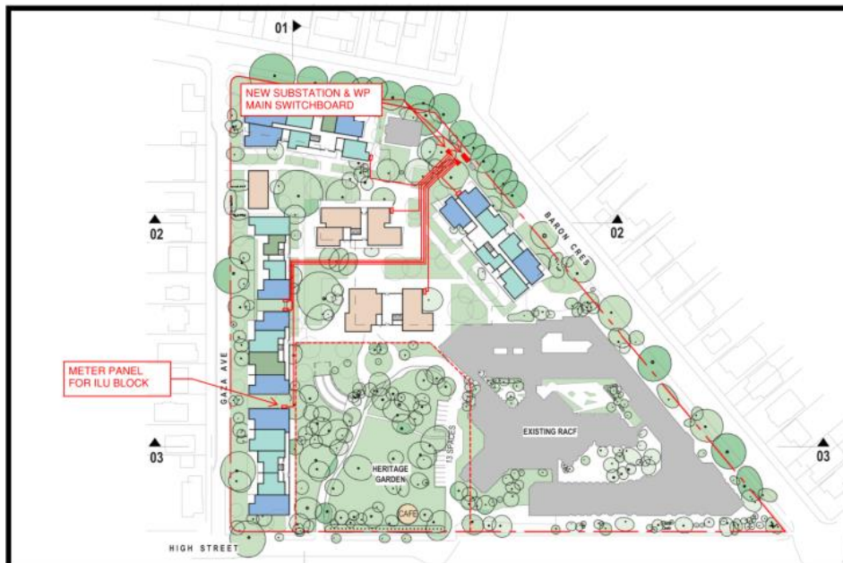
Figure 5.2 Proposed LV reticulation to new ILU Buildings
